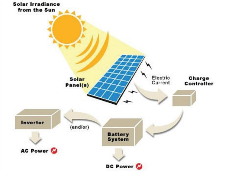
How a photovoltaic system works
